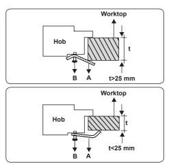
Important: If the appliance is to be installed above a cupboard or drawer it is absolutely essential that you place a separator between the base of the appliance and the drawer unit.
